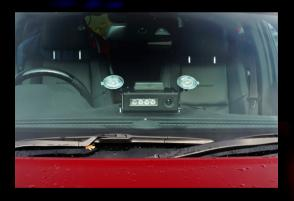
At it's base level the ANPRnow camera can be used for data gathering, requiring no input or action by the driver. A single windscreen camera can read multiple lanes at once.
