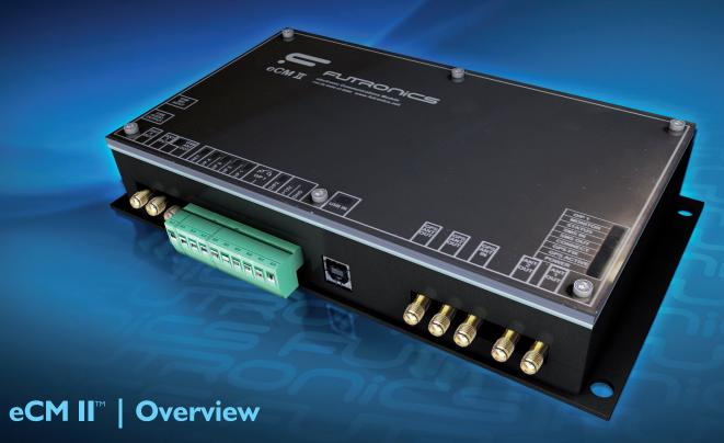
The **Futronics eCM II** is an incredibly versatile communications and GIS module, designed to provide robust communications, remote diagnostics and geographical information between mobile or static systems and a control room. Remote users can quickly determine location, equipment status and system performance metrics, using the **eCM II** integrated GPRS diagnostics feature, and where necessary send command and control signals.
